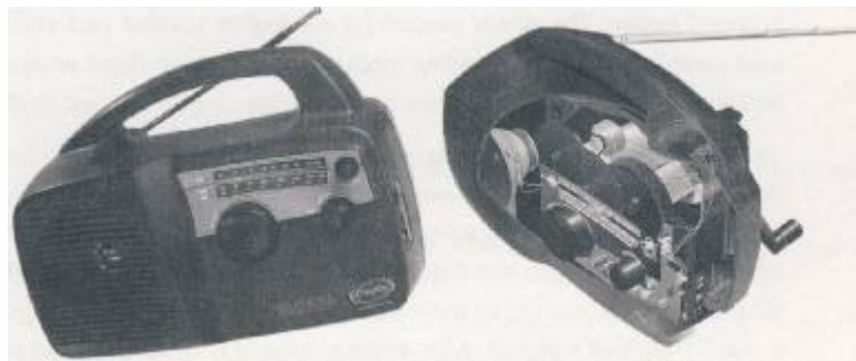
Figure 8.21 The Freeplay Radio: product image and internal schemata. (Reprinted with permission of Freeplay Group.)
